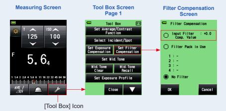
4. Input the compensation value on the Filter Comp. Value Screen. (See → P11 for details about how to input the value.)
