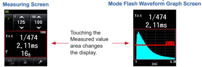
\* The Graph Screen cannot be used to make measurements.
