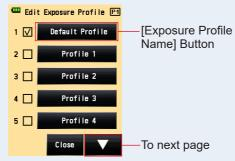
3. Touch the [Exposure Profile Name] Button on the Edit Exposure Profile Screen.
