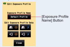
6. Touch the icon for the desired light receiving method and light source in "Edit Exposure Profile Data" on the Edit Exposure Profile Screen.
