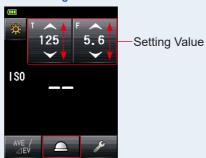
**6.** Press the Measuring Button **6** to measure the light on the side of the meter.
