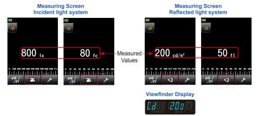
\* If the light receiving method is changed from the incident light system to the reflected light system, the display is automatically changed from the Ambient Light Illuminance (Ix or fc) Mode to the Ambient Light Luminance (cd/m² or fl) Mode.
