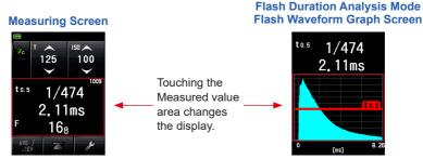
\* The Graph Screen cannot be used to make measurements.
