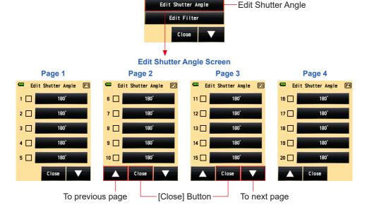
1. Press the Menu Button 9 on the meter to open
